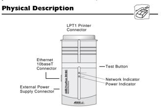
Installing AXIS PrintPoint 140 BJC
